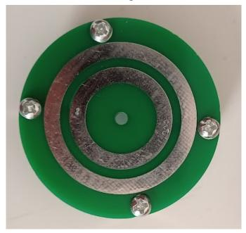
**Step 8:**Fasten the lower circuit board to the motor shaft with an M3 screw (10 mm).
