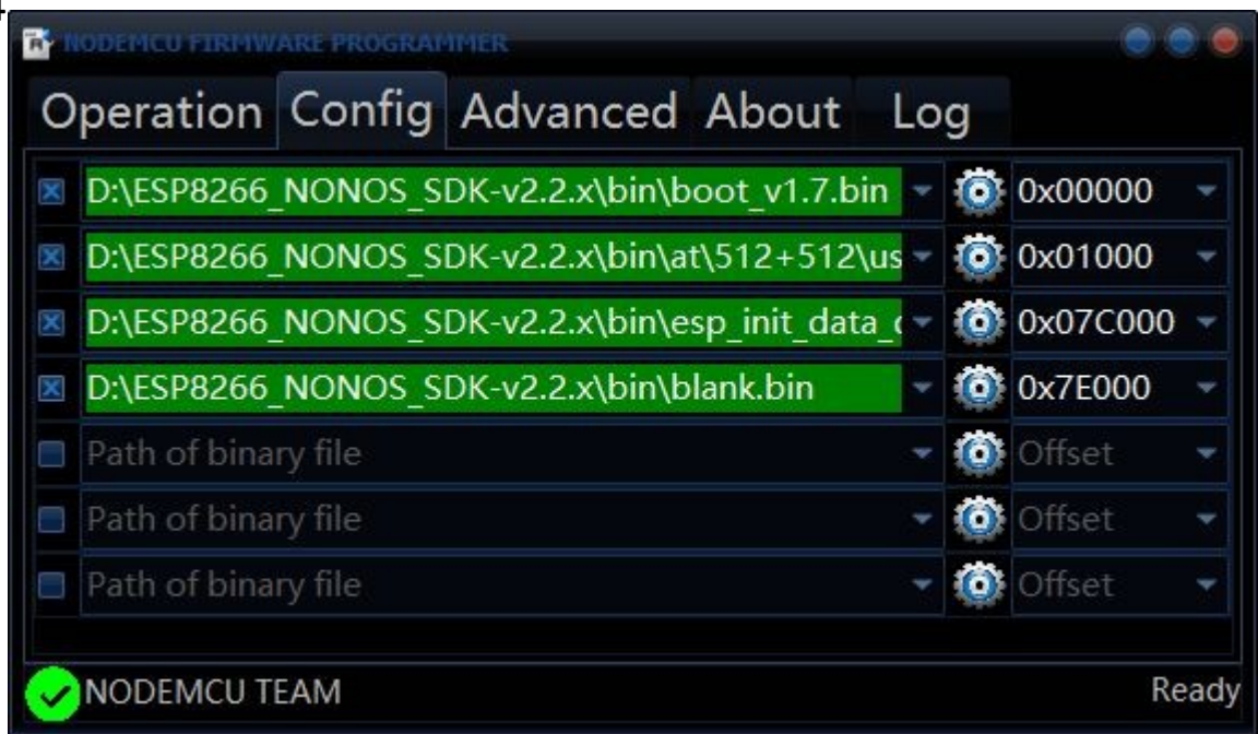
fig. 7.3.2 -Configuration of the NodeMCU Flasher
