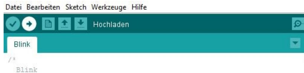
fig. 6.5.2.2 Starting the compilation and transfer process of the code to the controller
