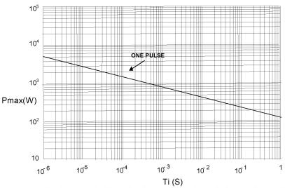
Maximum permissible peak pulse power(Pmax) as a fuction of pulse duration(T) Condition test: Resistance change  $\leq \pm 5\%$  with pulse 1000 cycles as like the figure.(Reference Only)
