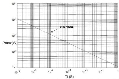
Maximum permissible peak pulse power(Pmax) as a fuction of pulse duration(Ti)
