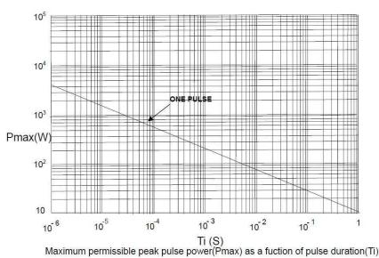
Condition test: Resistance change ≤ ±5% with pulse 1000 cycles as like the figure.(Reference Only)
