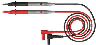
H3001 Probe: Length 130mm, Tip Φ2mm Plug: Φ4mm Cross Plug, right angle type Wire: 20AWG, red/black Length: 1000mm Safety Class: EN61010-031, 1000V CATIII/600V CATIV, MAX 10A
